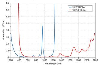
Typical values are shown. Note that 1 dB/m corresponds to 21 % loss per meter. So for example the blue peak at 950 nm means a transmission dip of about 20 % for a 1 meter fiber.
